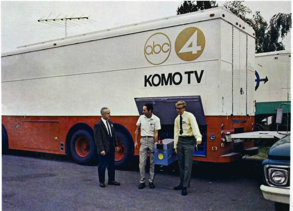
Left to right, Ralph Mifflin, Wally Schutter, and John Carlborn carrying one of the RCA TK-44A cameras by means of convenient fold-out handles located on either side. The truck skirt compartment in the background houses two power driven camera cable reels as does the compartment directly forward of the truck rear wheels. A similar compartment on the opposite side contains shock mounts for six TK-44A cameras.
