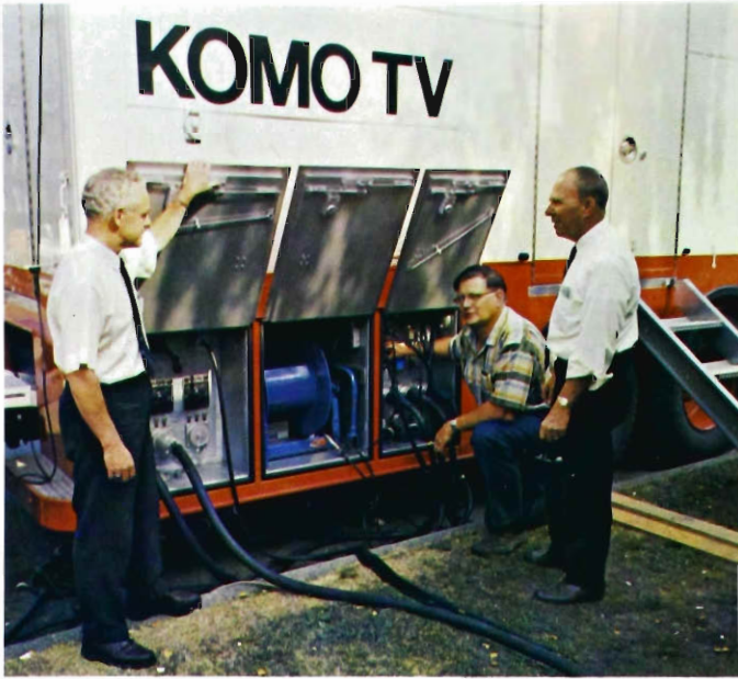
Left to right, Ralph Mifflin, Wally Schutter, and John Carlborn carrying one of the RCA TK-44A cameras by means of convenient fold-out handles located on either side. The truck skirt compartment in the background houses two power driven camera cable reels as does the compartment directly forward of the truck rear wheels. A similar compartment on the opposite side contains shock mounts for six TK-44A cameras.
